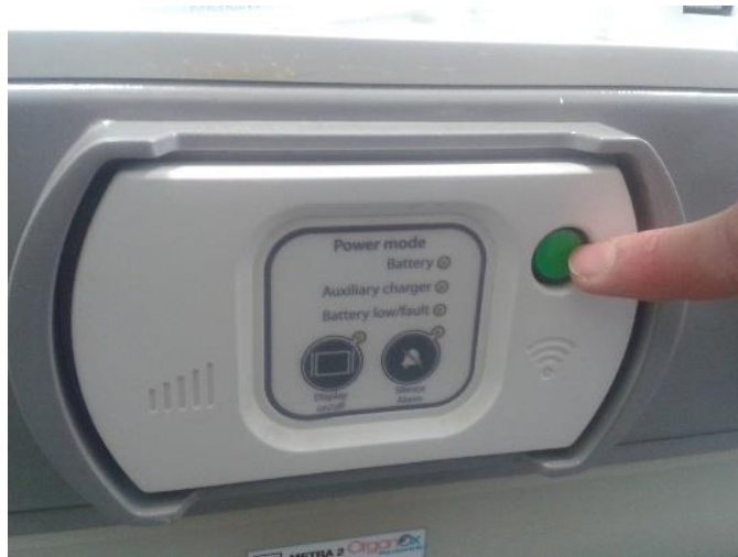
The position of the Wi-Fi on/off button
